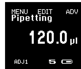
The pipette is set to use the adjustment values saved to ADJ1.
