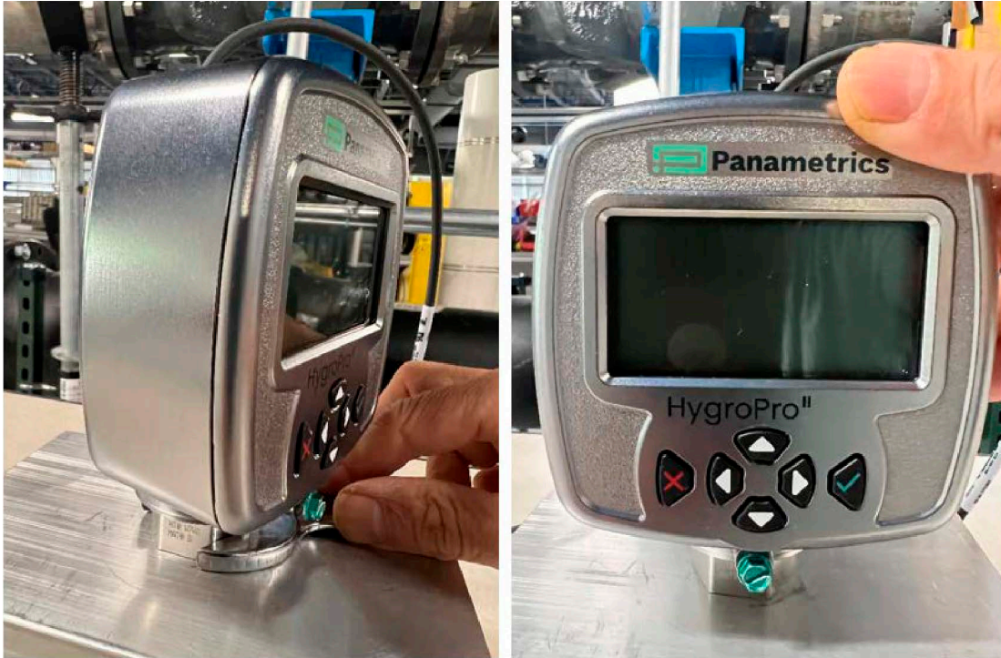
Figure 6: HygroPro II installation step 3 – installing into sample cell
