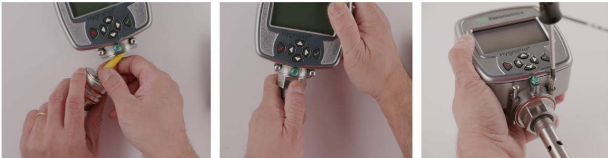
Figure 19: Reinstalling the Hygro II RTE probe into the dismantled transmitter
