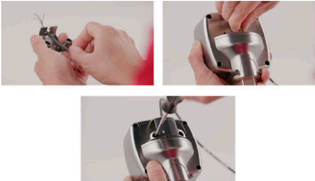
Figure 4: HygroPro II installation step 1 – initial wiring
