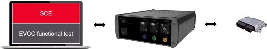
Figure 2. Development tests of EVCC with Com Tester and Smart Charging Emulation Software (SCE)
