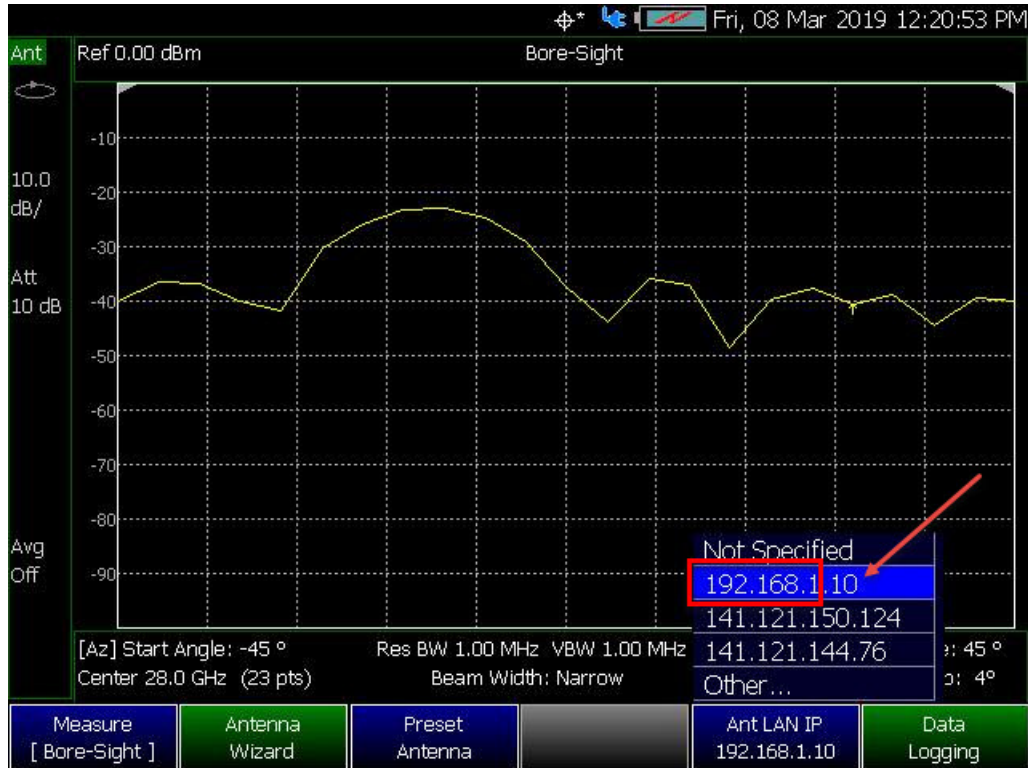
Figure 14-15 Example of Phased Array Antenna and FieldFox Static IP Setup - First Three Static IP Fields Are the Same
