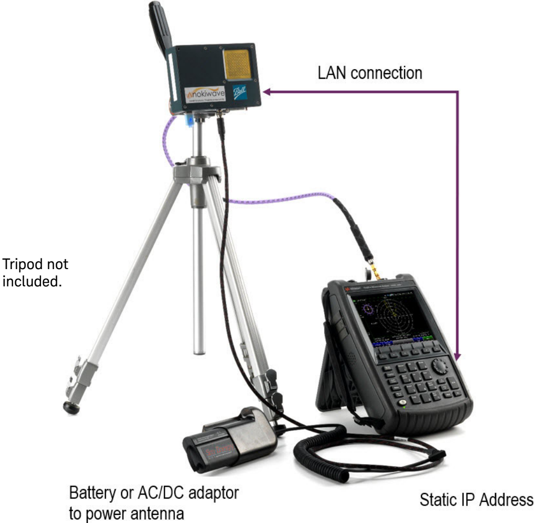
Figure 14-1 Example of local point-to-point LAN connection
