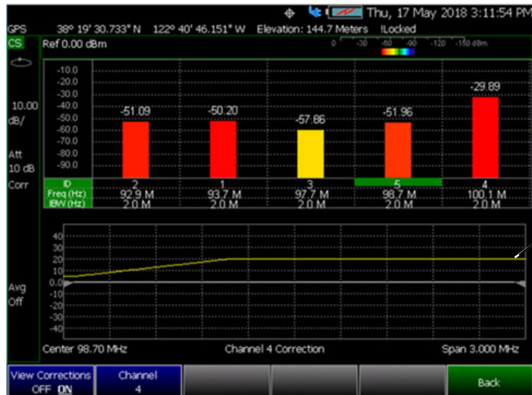
Figure 28-22 Yellow Trace with Cable and Antenna Corrections
