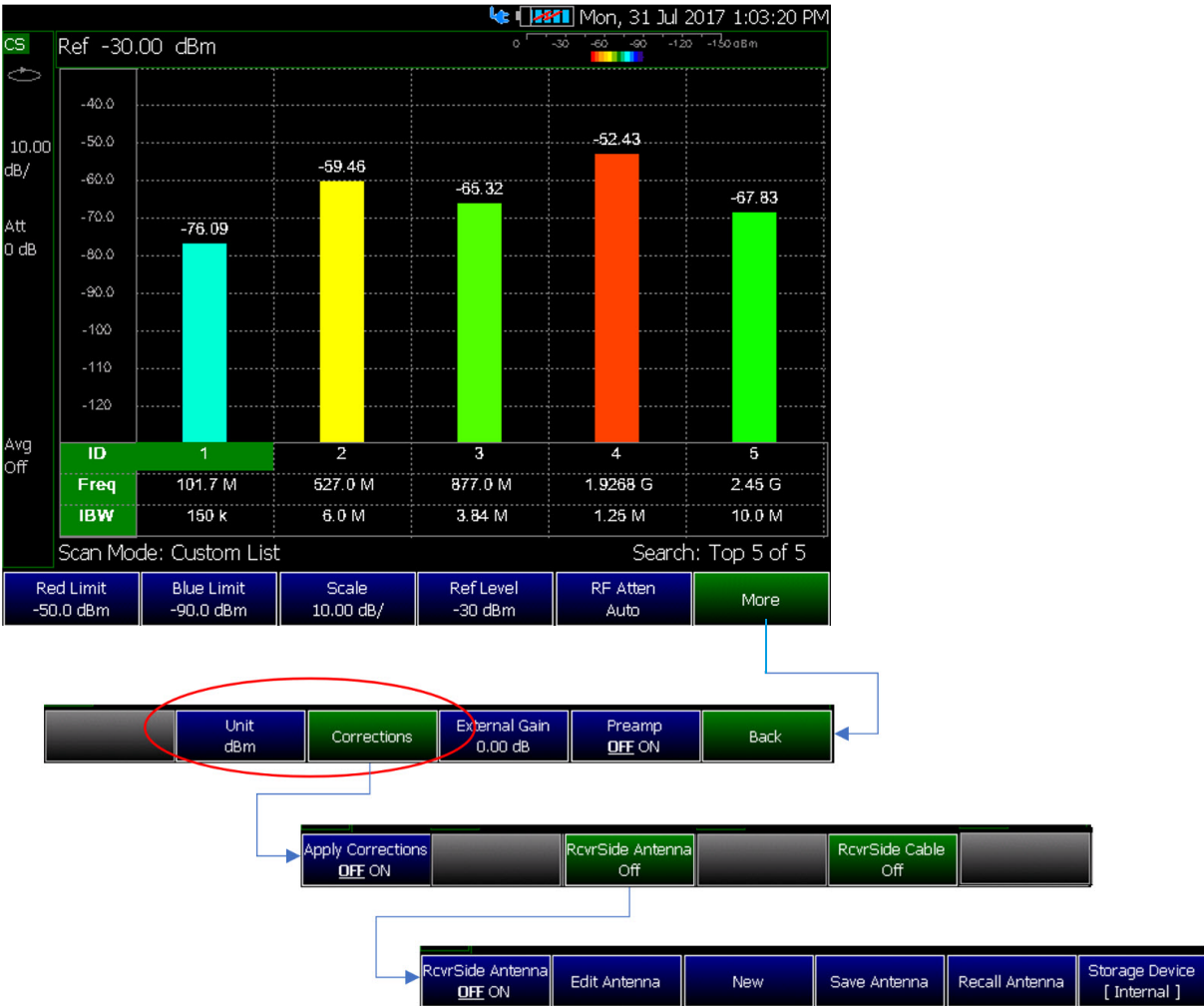
Figure 28-20 Overview of Field Strength for Channel Scanner (See also, Figure 28-21 on page 674. )
