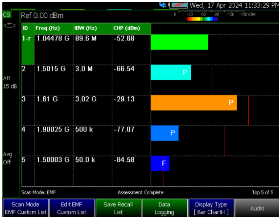
Figure 28-9 Bar Chart Horizontal Display Type - EMF Custom List with Limit Line Configured
