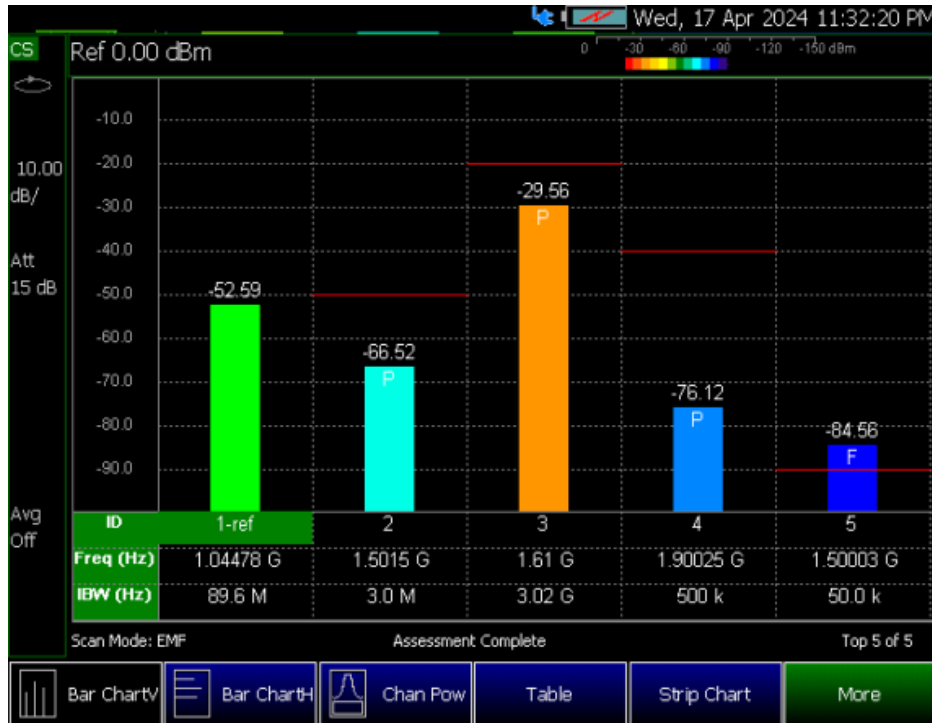
Figure 28-7 Bar Chart Vertical Display Type - EMF Custom List with Limit Line Configured
