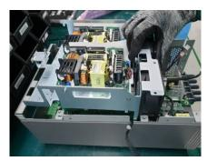
Remove 14 screws from the PCA mainboard using a T10 bit.
