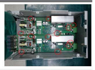
Lift and remove the the two PCA mainboards from the chassis.
