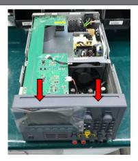
**7** Detach the mainboard connector from the IO board.
