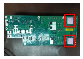
20 Remove two screws from the IO board using a T10 bit.
