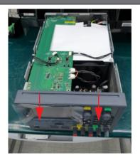
**8** Detach the power PSU connector from the IO board.
