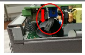
**12** Remove the GPIB module from the chassis.
