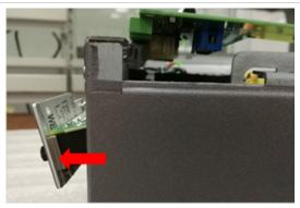
**13** Detach the AC inlet connector from the PSU module.
