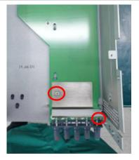
Remove three screws from the IO board using a T10 bit. Remove the IO board from the chassis.
