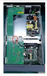
**8** Detach the power PSU connector from the IO board.
