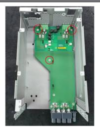
22 Unsolder the binding post assembly from the IO board. Remove the four screws with a T-10 bit. Replace the existing binding post assembly with a new binding post assembly.
