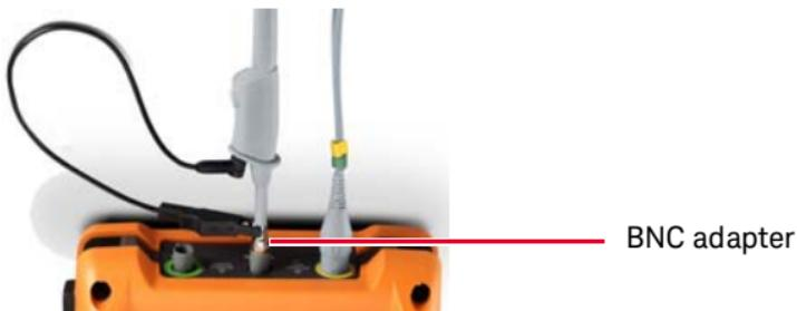
Use a nonmetallic tool to adjust the trimmer capacitor on the probe for the flattest pulse possible.
