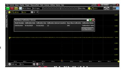
Import your instrument's calibration status document from the main PCA screen. Or, use PCA to access calibration certificates and test reports with a link to the online Keysight Support Portal (support.keysight.com).
