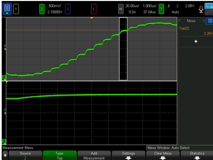
Figure 48 Isolating area for Top measurement
