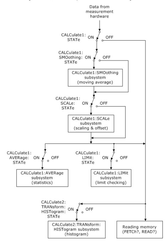
The CALCulate1 subsystem is enabled or disabled by the CALCulate1:STATe command. If CALCulate1:STATe OFF is set, no calculations are performed on the measurements, and the measurements will flow directly to the reading memory.
