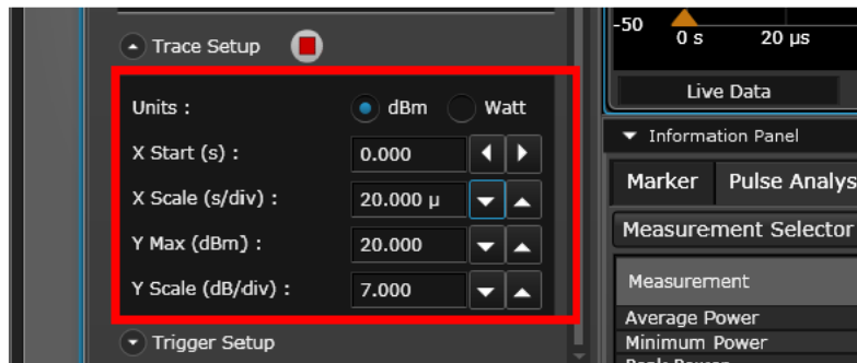
Figure 2-13 Setting the trace scales
