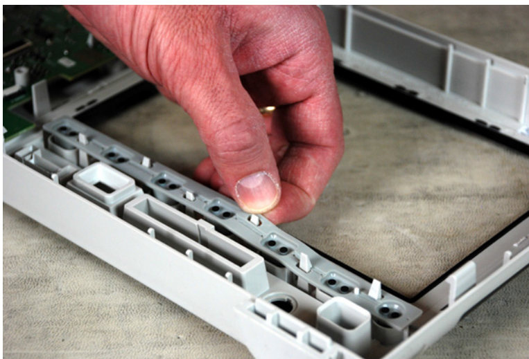
Figure 42 Remove the softkey keypad from the bezel
