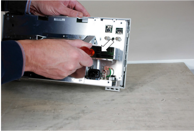
Figure 25 Removing the option module guide to acquisition board screw
