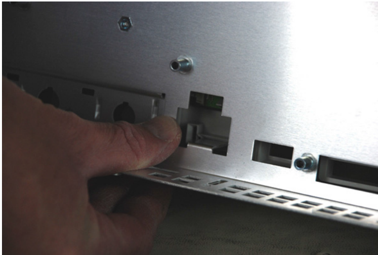
Figure 37 HINT: When reinstalling bezel, align ground terminal first
