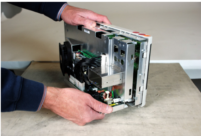
Figure 28 Separating the rear and front decks
