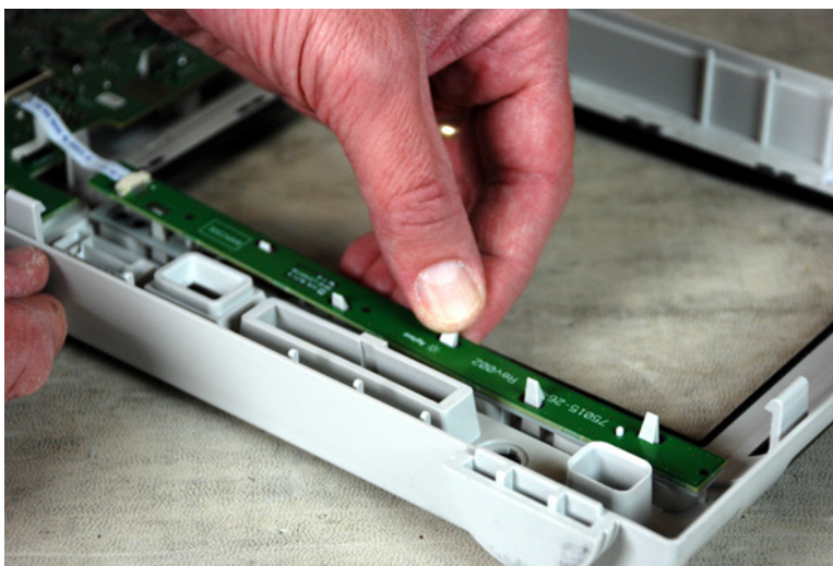
Figure 41 Unclip the softkey board from the bezel
