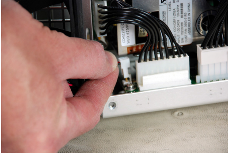
Figure 51 Disconnecting fan power cable
