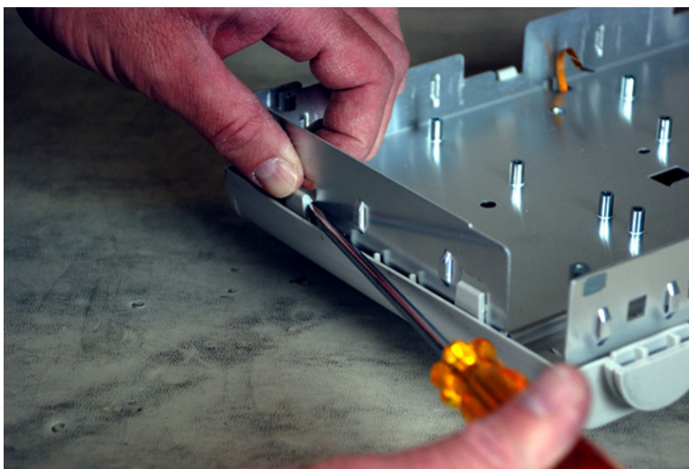
Figure 35 Release the bezel clips from the front deck
