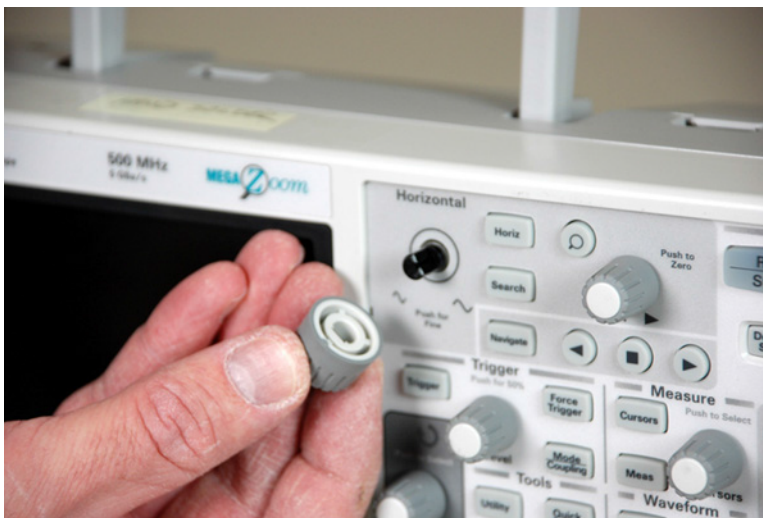
Figure 14 Removing the front panel knobs
