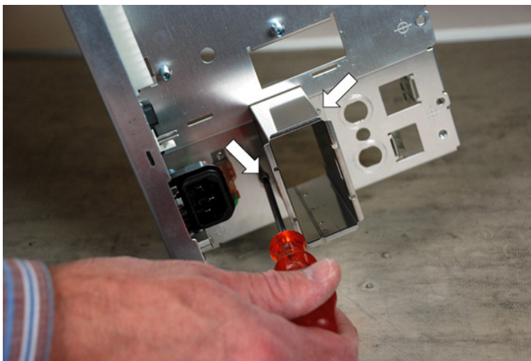
Figure 57 Removing the option module guide
