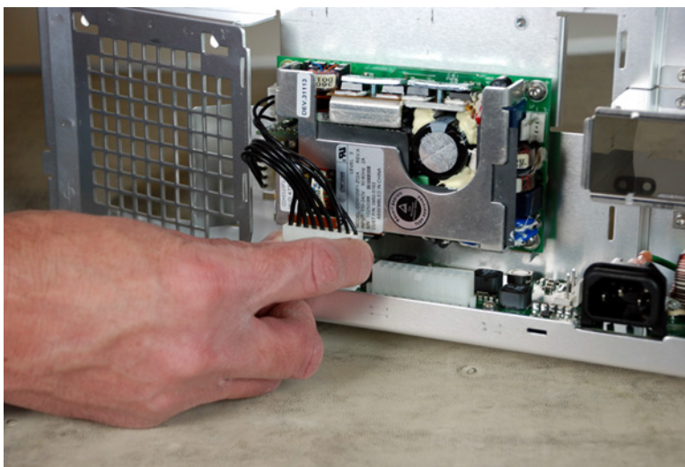
Figure 55 Disconnecting the DC cable from the line filter board
