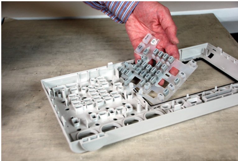
Figure 44 Remove the keyboard keypad from the bezel
