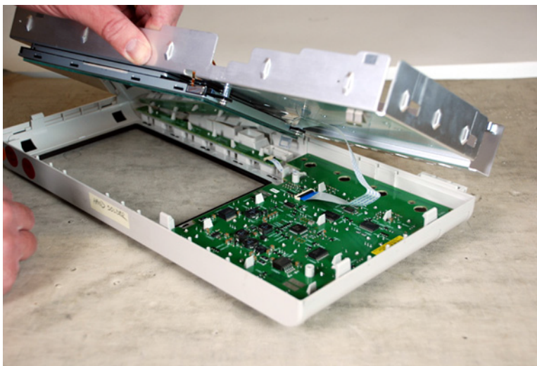
Figure 38 Gently lift front deck from bezel
