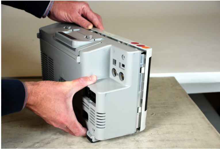
Figure 16 Removing bucket assembly
