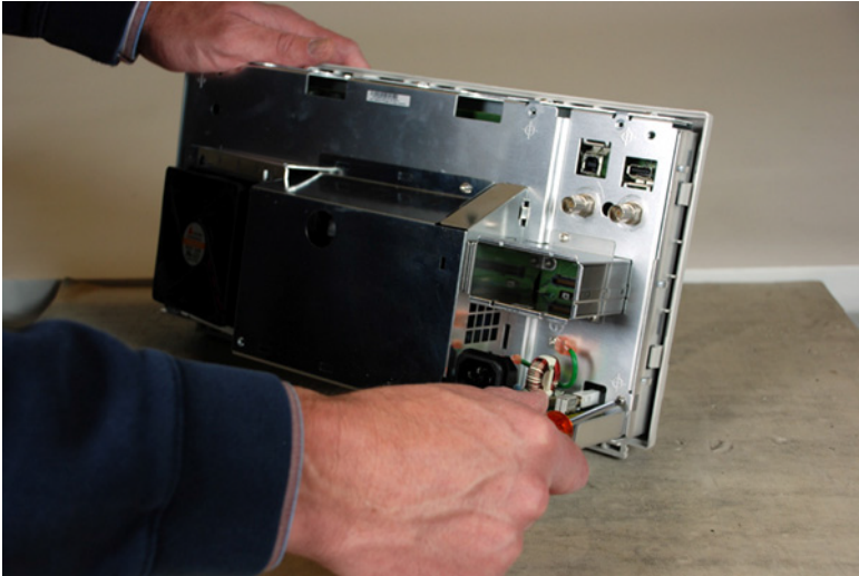
Figure 22 Removing the bottom right rear deck screw
