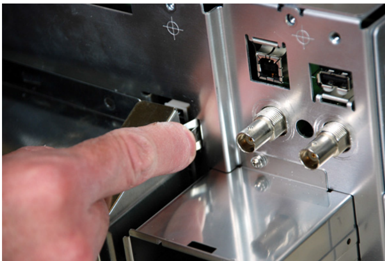
Figure 18 Unclipping the power supply shield right side
