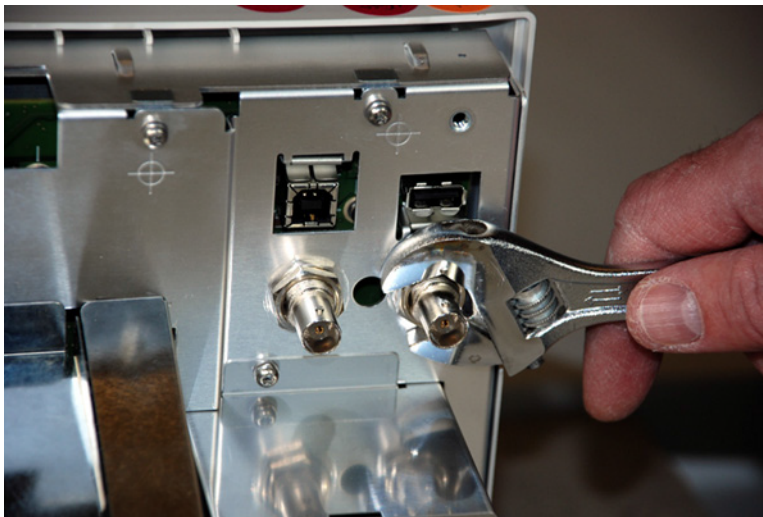
Figure 20 Removing the BNC nuts and washers
