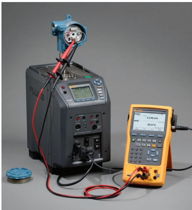
Figure 5. Fluke 754 and Fluke Calibration 9144P dry-well calibrating a 4-20 mA transmitter and temperature sensor.
