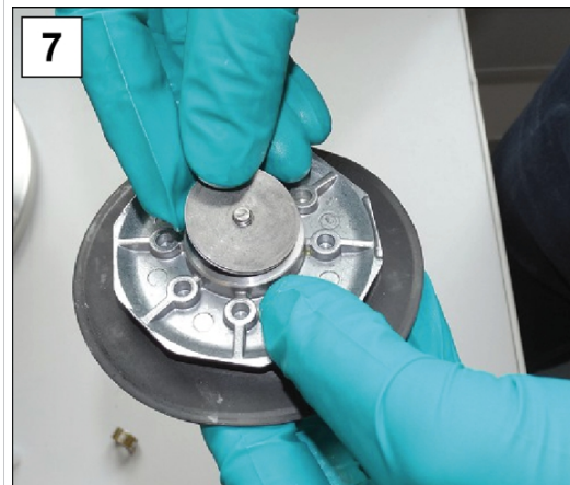
7. Place all spacers onto the threaded bolt.
