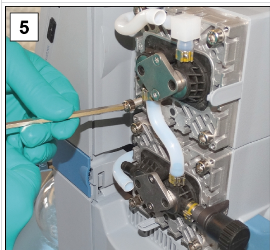
3. Open the hose clamps of the outer hoses. Flat-head screwdriver size 1.
