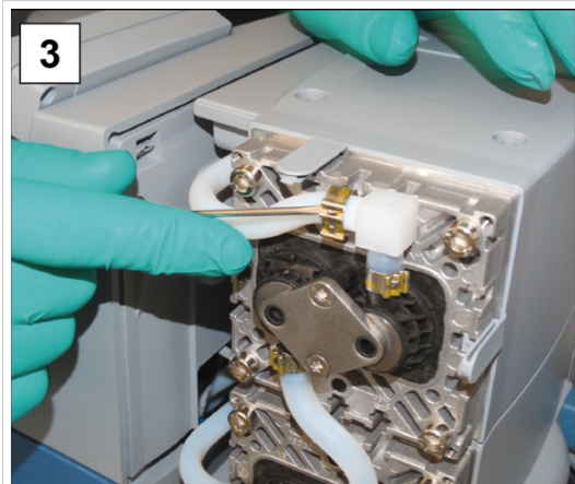
3. Open the hose clamps of the outer hoses. Flat-head screwdriver size 1.
