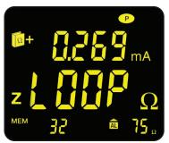
Detects and displays possible false readings associated with metal loops
