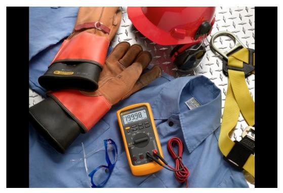
Depending on the task, basic PPE for solar PV technicians can include gloves, hard hat and ear protection, safety harness, arc-rated clothing, and a Fluke 87 V Industrial Multimeter.
