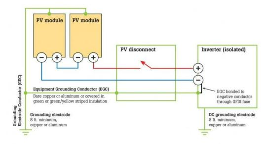
Figure 1: Negatively-Grounded PV System (DC Side)
