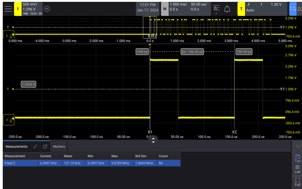
Figure 40 Isolating an event for Frequency measurement
