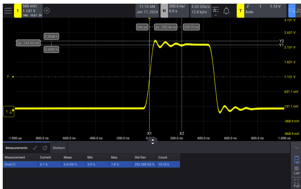
Figure 39 Automatic Overshoot measurement
