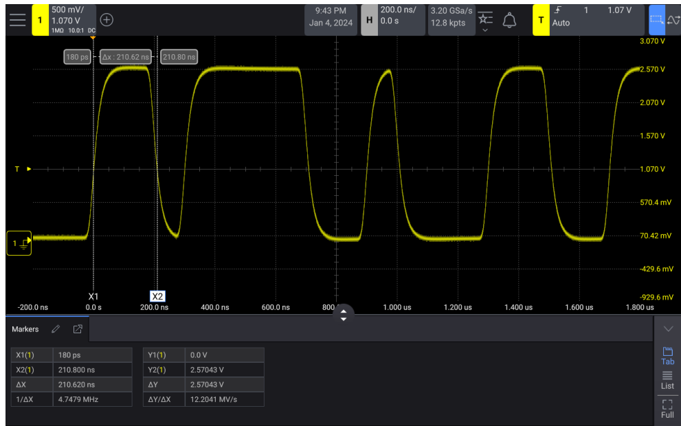
Figure 36 Measuring pulse width with markers
