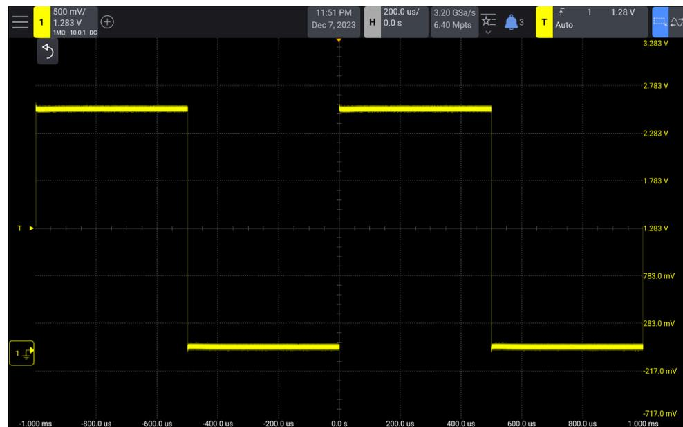
If you see the waveform, but the square wave is not shaped correctly as shown above, perform the procedure **"To compensate passive probes"** on page 57.
