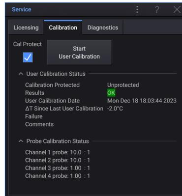
Note that passive probes do not need to be calibrated, but InfiniiMax probes can be calibrated.
