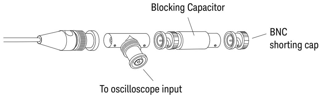
**Figure 4** Using a Blocking Capacitor to Reduce Noise
