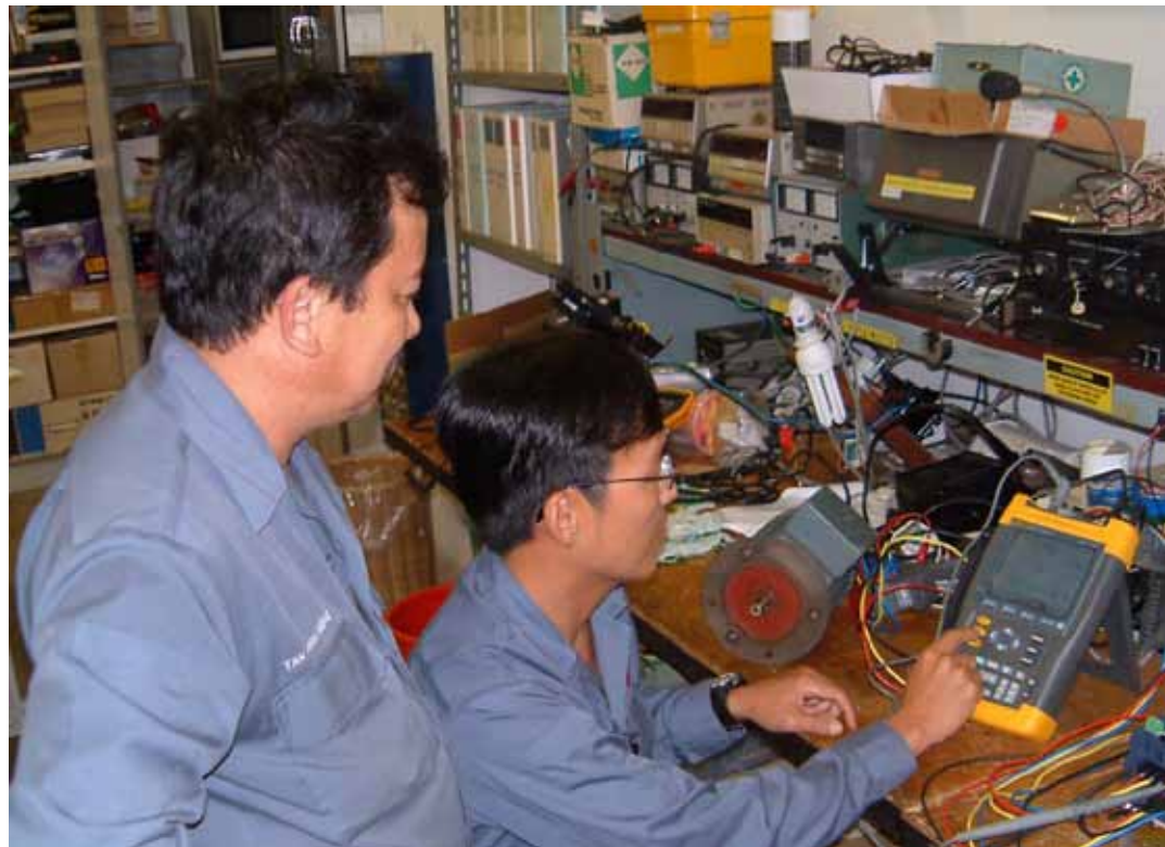
Mr. Tan and Mr. Awyong make measurements of the speed drives using the Fluke 192 ScopeMeter.
