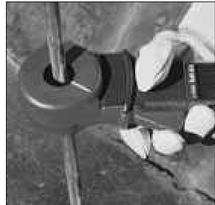
Large inner jaw diameter fits rods and conductors up to 1000 MCM
